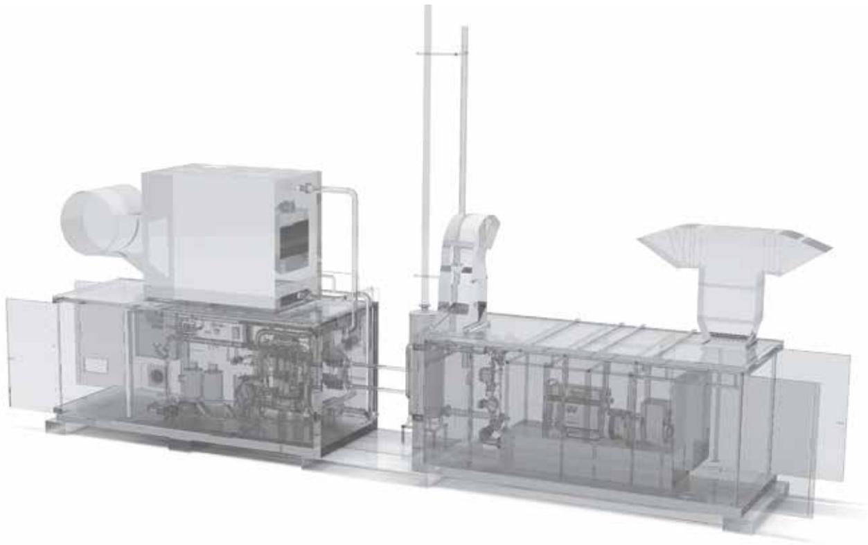
Modular construction of CHP and absorption chiller containers
